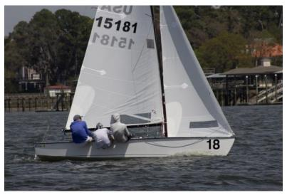
When perfectly set up in every condition there should be visible diagonal wrinkles in the lower ¼ of the main, from the mast towards the clew. These wrinkles should start just behind the mast and stop ½ back on the boom. In the Backstay section we will describe how these wrinkles are the ideal
