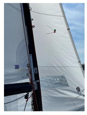
The "groove" refers to that area where the boat feels the most comfortable sailing upwind. The lower end of the groove, when both the windward and leeward jib luff tell tales flow, is when the boat is building speed and power. Acceleration, punching through waves, rolling out of a tack are all times when both telltales should stream.
