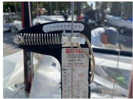
With the blocks in place, the lowers close to 300 lbs., the uppers will drop to 165-190lbs-17-19 AND there will be  $1 \frac{3}{4}$ "-2" of prebend at the spreaders. (Pulling the main halyard down to the gooseneck and checking the distance from the wire to the back of the mast at the spreaders will help gauge the proper prebend.)
